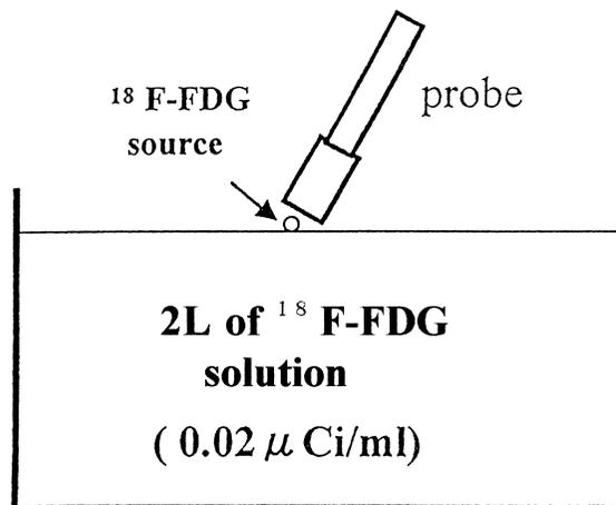
**Fig. 4** For simulation relevant to abdominal surgery, a  $^{18}\text{F}$ -FDG source was placed on the surface of the background solution. Counts were measured by positioning the probe to contact the source.
