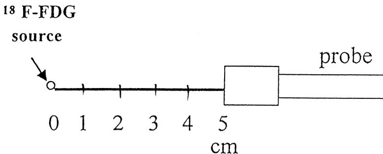
**Fig. 2** Counts were measured for source-to-probe distances ranging from 0 to 5 cm.
