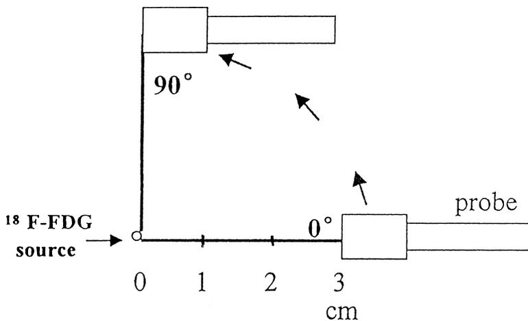
**Fig. 3** Angular sensitivities were measured for source-to-probe angles between 0 and 90 degrees.
