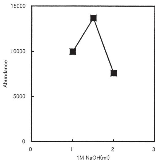
**Fig. 2** Effect of 1N NaOH volume on extraction rates in HS-SPME. Each extraction was performed for 15 min at 100°C from a 50 mg rat hair sample spiked with p,p'-DDE at 2.0 ng/mg. Pre-heating time = 0 min.
