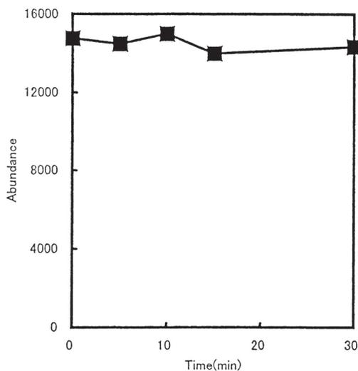
**Fig. 4** The effect of pre-heating time on extraction rates in HS-SPME. Each extraction was performed for 15 min at 140°C from a 50 mg rat hair sample spiked with p,p'-DDE at 2.0 ng/mg and 1.5 ml 1N NaOH.
