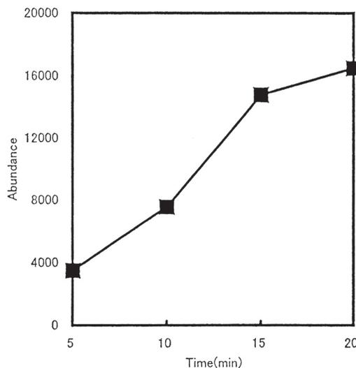
**Fig. 5** The effect of exposure time on extraction rates in HS-SPME. Each extraction was performed at 140°C from a 50 mg rat hair sample spiked with p,p'-DDE at 2.0 ng/mg and 1.5 ml 1N NaOH. Pre-heating time = 0 min.
