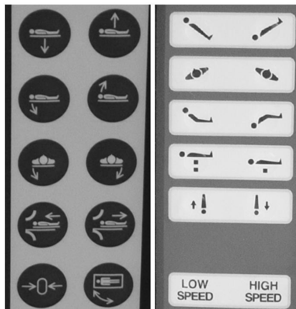
Fig. 4. Left: Controller for a conventional operating table. Right: Controller for the newly developed flexible operating table. With both tables, the patient can be positioned in trendelenburg or reverse trendelenburg, rotated to the right or left, and elevated or lowered. Note that the controller for the newly developed flexible operating table includes buttons than are used to bend the table, which is not possible with the inflexible operating table (left).
