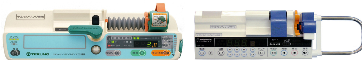
Fig. 1 Features of Two Different Pumps. Type A: TE-331S0N (Terumo Corporation): PFS syringe can be used without changing operational mode. Type B: CSP-100S (Daiken Medical Co., Ltd.): Operational mode must be changed before using PSF syringe. Type A (left): TE-331S0N, Type B (right): CSP-100S,
