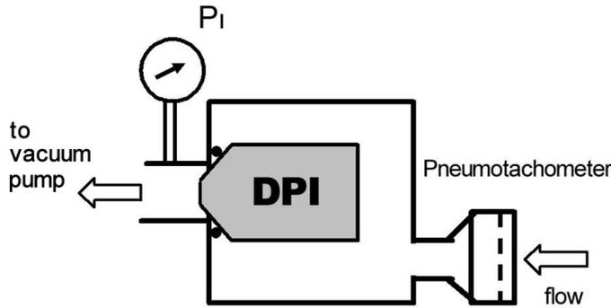
Fig. 1 The device was a tightly sealed box. A negative pressure was applied to one hole and a pneumotachometer was fixed to another hole. DPI: dry powder inhaler,  $P_1$ : inspiratory pressure.
