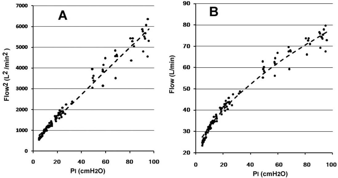
Fig. 2 Examples of  $P_1$  vs. flow<sup>2</sup> relationship (A) and  $P_1$  vs. flow relationship (B) of Twisthalers. All the flow points scatter below the regression curve (dashed curve) in the range below a certain  $P_1$ .  $P_1$ : inspiratory pressure.
