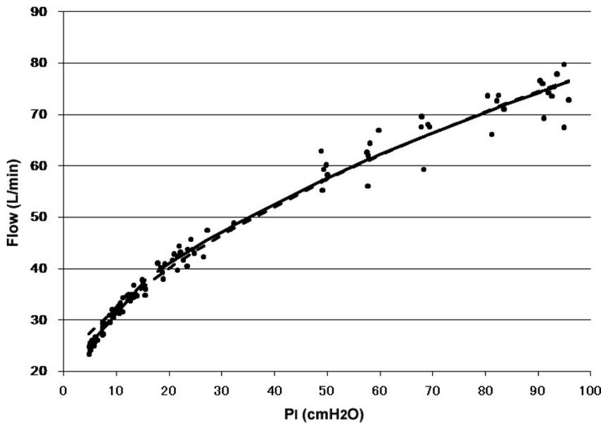
**Fig. 3** Comparison of the  $P_1$  - flow regression curves based on a parabolic model (dashed curve) and a biphasic model (solid curve) of Twisthalers.
