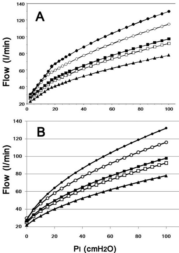
**Fig. 4** Simulated  $P_1$  vs. flow relationships of all DPIs based on parameters shown in Table 1. A: curves based on a biphasic model. B: curves based on a parabolic model (5).
