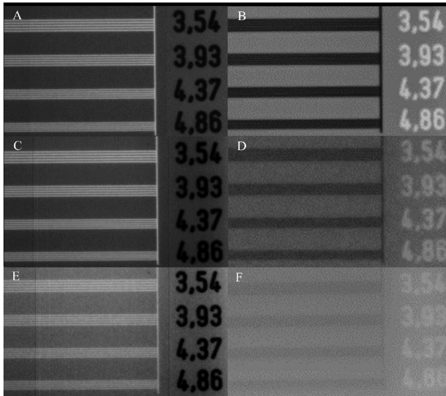
Fig. 2 X-ray test chart following various types of X-ray system exposure: A) Direct exposure to the cerium anode X-ray system. B) Direct exposure to the conventional X-ray system. C) Indirect exposure to the cerium anode X-ray system through a 10-cm-thick acrylic plate. D) Indirect exposure to the conventional X-ray system through a 10-cm-thick acrylic plate. E) Indirect exposure to the cerium anode X-ray system through a 20-cm-thick acrylic plate. F) X-ray test chart after indirect exposure to the conventional X-ray system through a 20-cm-thick acrylic plate.
