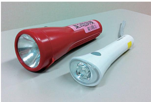
**Fig. 1** The torches used by the survey participants; a traditional yellow-light torch featuring a light bulb (left) and a white-light torch featuring a light-emitting diode (LED; right). The illumination intensity of LED torches is higher than that of traditional (i.e., non-LED) torches.
