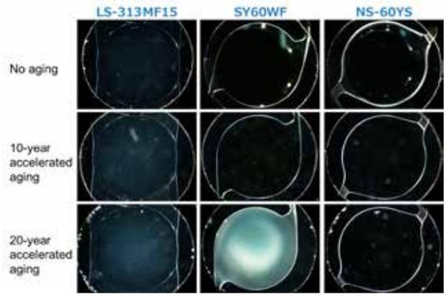
Fig. 2 Result of Dark-field appearance in water
